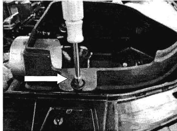
g) Secure the MOPAR Cold Air Box to the core support with the M6 bolt removed from step 2f).
